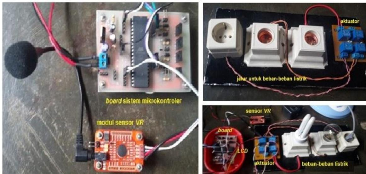
**Gambar 5** Penampang fisis *minimum system* terintegrasi
