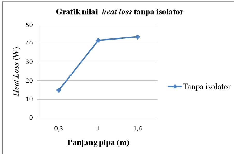
Gambar 1. Grafik nilai *heat loss* tanpa isolator
