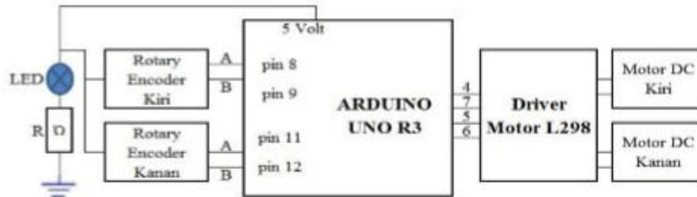
Gambar 3. Pengujian Rotary Encoder
