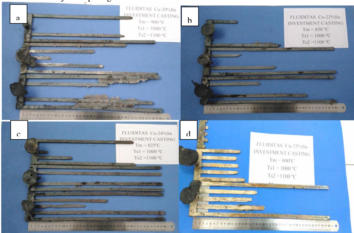
Gambar 6. Uji fluiditas investment casting (a) 20%Sn (b)22%Sn (c)24%Sn (d) Cu-25%Sn
