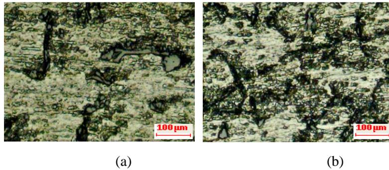
**Gambar 4. Foto mikro matriks (a) Al7Si (b) Al7Si1Mg**
