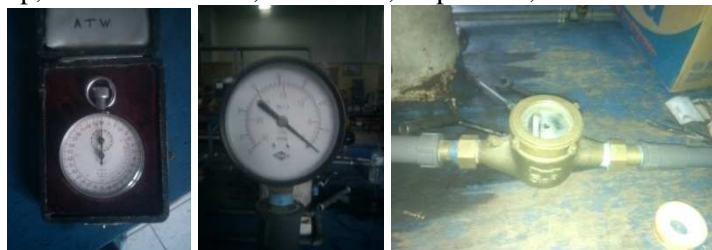
Gambar 3 alat ukur Stop watch diamond, manometer hisap dan flow meter
