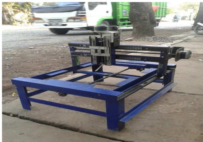
**Gambar 4. Prototipe Mesin Cnc Router PCB**
