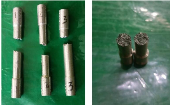
Gambar 6. Patah getas paduan Al-4,4%Si-Cu
