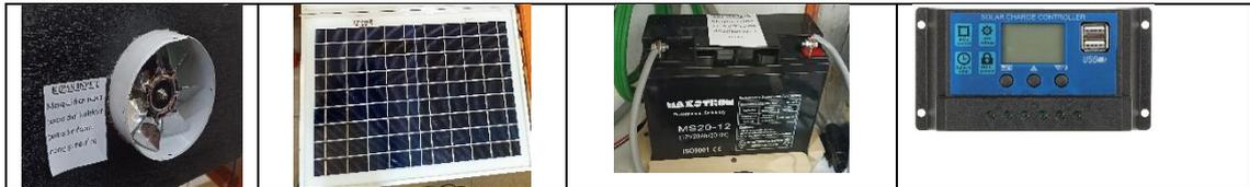
**Gambar 7. Kipas 20W, PV 10 Wp, Baterai 12V 25Ah, dan SCC 30 A.**
