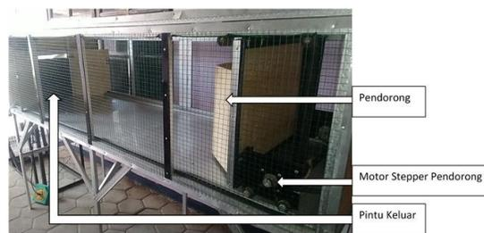
**Gambar 3.3. Hasil Alat Sistem Panen Ayam Pedaging Secara Otomatis Dari Tampak Belakang**
