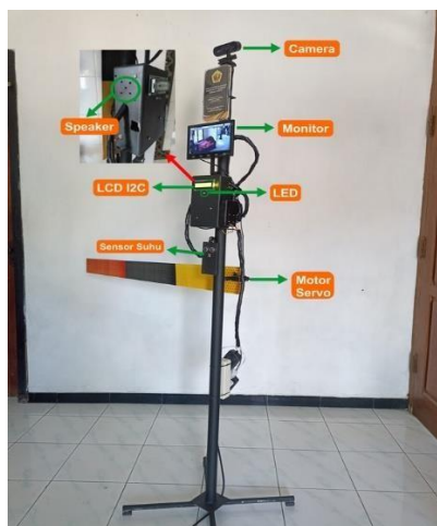
Gambar 6. Hasil Alat Mask Detector Gate System
