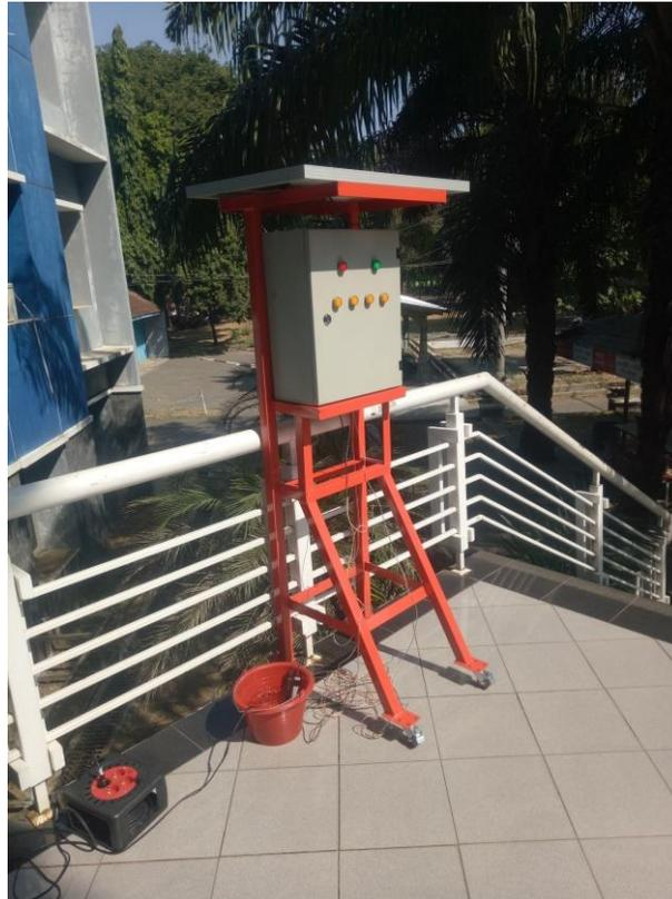
Gambar 10. Alat Monitoring Kuat Arus, Tegangan Dan Daya
