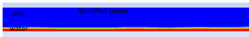
Gambar 5. Hasil Simulasi Aliran Stratified Smooth ( J_L = 0,025 m/s, J_G = 1,88 m/s, dan \phi = 19 mm )
