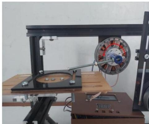
**Gambar 4. Uji Beban Motor Servo**
