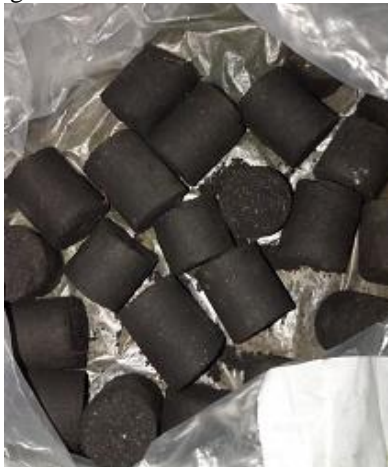
Figure 2. Result of briquette made of sawdust and corncob
