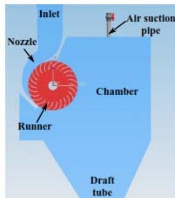
Gambar 3. Skema Model Turbin Crossflow
