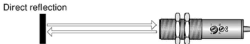
Gambar 1. Sensor *Photoelectric Direct Reflection*
