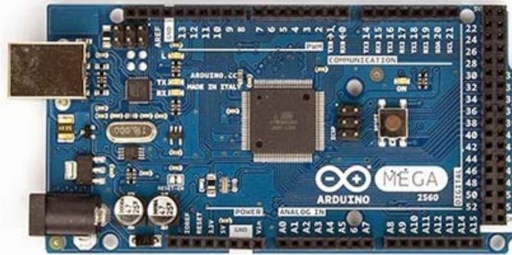
**Gambar 2. Board Arduino Mega 2560 [4]**
