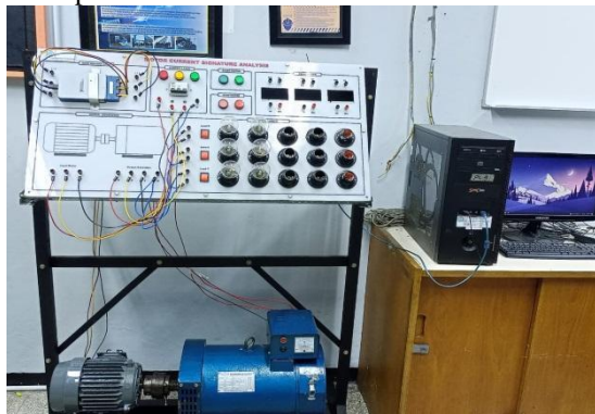
Gambar 3. Implementasi sistem deteksi kerusakan inner race bearing .
