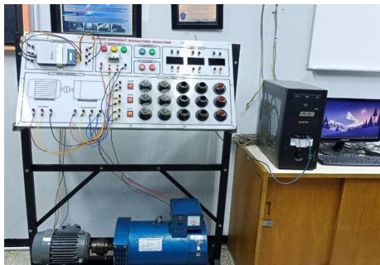
Gambar 3. Implementasi sistem deteksi kerusakan inner race bearing .
